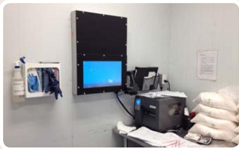
This photo was taken from one of the dispensing rooms at GFR. The black box on the wall is a computer with a touch screen embedded. This box is dust proof and waterproof, connected to a Datamax label printer and it has a Wireless scanner attached to it.
