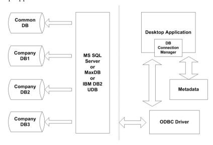
Figure 2: Server Component Architecture
